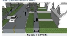
To ensure a more user-friendly and accommodating experience for all, bicycle and pedestrian facilities should be separated. In a reas with higher bicycle use or where separated bicycle facilities are not provided, a sidepath should be included.
